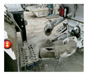
A driver suffered a restricted duty injury when discharging into a large concrete pump. The driver was standing on the first step of the ladder when the discharge pipe on the pump blew out and caused high pressure concrete to hit the driver in the chest causing bruising to the chest area. Fortunately, the driver had on all his personal protective equipment including his face shield which helped avoid further injury.
